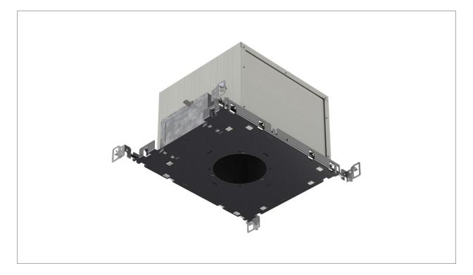
The 2-010 series housing is designed for insulated and airtight ceilings. Performing in accordance with ASTM E283-91, the airtight option also meets the requirements of "having no more than 2.0 CFM air movement from the conditioned space to the ceiling cavity" (Sec. 502.4 of 1991 WSEC—Washington State Electrical Code).
