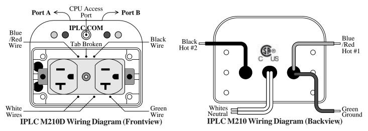
Electrical & Wiring Specifications: Dual 125 VAC, AC supply, 20 Amps rms, 60 Hz circuit operation, resistive loads only. 240 VAC single phase split circuit with neutral, 208 VAC Line-to-Line 3 phase with neutral. \*please refer to IPLC M210 wiring diagram BACKVIEW (shown above) and table (shown below).
