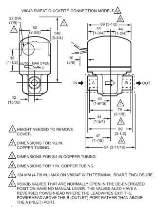
A OPENING FOR 1/2 IN. CONDUIT ON MANUAL LEVER SIDE FOR V8043 MC23257 Two-way on-off low voltage valves consist of an actuator and valve assembly for controlling the flow of hot water.
