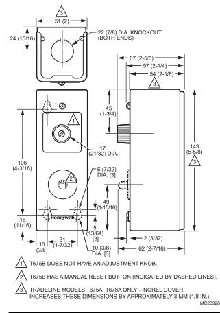
Remote bulb thermostats regulate temperature of air or liquids in ducts, pipes, tanks and boilers.
