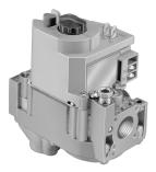
Type: Single Stage Body Pattern: Straight-through Type of Gas: Natural Capacity: 130,000 BTU/hr 1 in. PD; 20,000 BTU/hr minimum 200,000 BTU/hr maximum Anticipator Setting: 0.5 A Ignition Type: Standing Pilot Pressure Ratings: 1/2 psi (3.5 kPa) Pressure Tapping: 1/8 in. NPT with plug Ambient Temperature Range: 0 F to 175 F (-18 C to +79 C)
