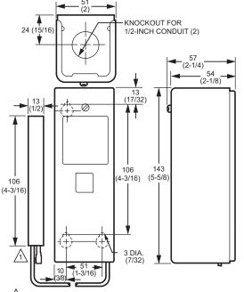
BULB LENGTH IS 91 (3-9/16) ON 15 TO 75 C AND 55 TO 175 F RANGE MC2388 For modulating control of water or air temperature in ducts, tanks and similar applications.
