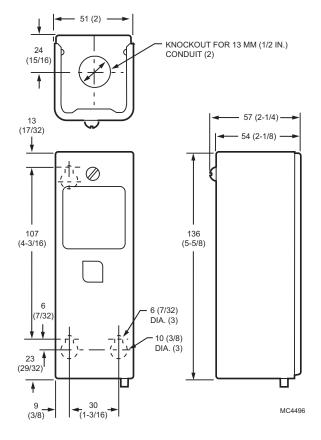
Provide limit or temperature control in refrigerated areas where remote mounting of sensing element is required.
