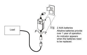
**NOTE**: To set the timer, it is not necessary to plug it in an electrical outlet.
