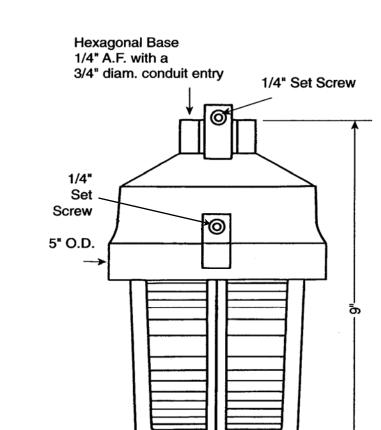
Guard 6 Ribs Equally Spaced
