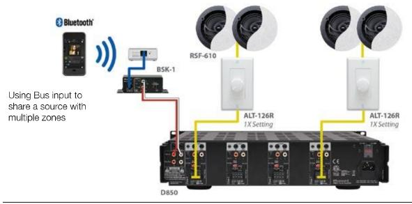
NOTE: Special wiring required when using Volume Controls with Impedance Matching. Log in to the Russound Tech Portal at russound.com for Tech Tips.
