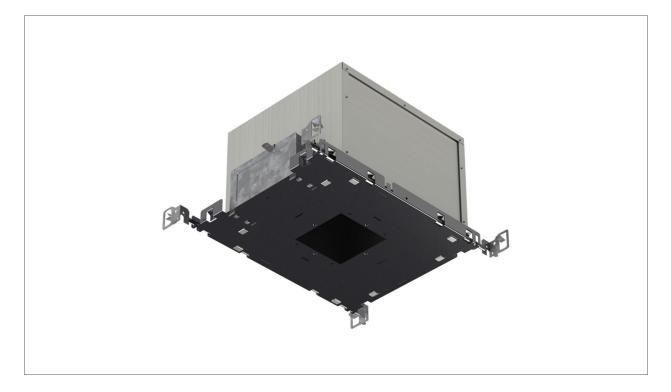
The 2-015 series housing is designed for insulated and airtight ceilings. Performing in accordance with ASTM E283-91, the airtight option also meets the requirements of "having no more than 2.0 CFM air movement from the conditioned space to the ceiling cavity" (Sec. 502.4 of 1991 WSEC—Washington State Electrical Code).
