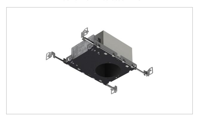
The D4B-F-R series is designed for non insulated ceilings. A unique design allows installation of very shallow plenums as low as 5" (when used with a shallow cover). A black powder coated 20 Ga. baseplate is designed for bidirectional mounting of hanger bars. A 18 Ga. galvanized steel junction box with multiple K.O. for easy wiring entry. The housing series is approved for branch circuit wiring.
