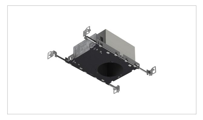
The D4X-F-R series is designed for non insulated ceilings. A 20 Ga. Black powder coated rolled steel baseplate is designed for bidirectional mounting of the hanger bars. 18 Ga. galvanized steel junction box with multiple K.O. allows for easy wiring entry. The series is approved for branch circuit wiring.
