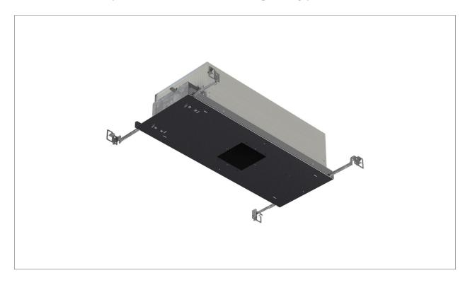
The D4B-IC1A-S series housing is designed for insulated and airtight ceilings. A black powder coated 20 Ga. cold rolled steel baseplate with a 18 Ga. galvanized steel junction box with multiple K.O. allows for easy wiring entry.Perfoming in accordance with ASTM E283-91, the airtight option also meets the requirements of "having no more than 2.0 CFM air movement from the conditioned space to the ceiling cavity" (Sec. 502.4 of 1991 WSEC- Washington State electrical code).
