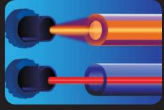
LED spot size: >100 $\mu$ m, 62.5/125 fiber. Laser spot size: ~30 $\mu$ m, 50/125 fiber.
