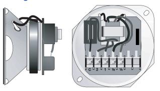
Desired wattage is selected by wiring into the corresponding terminal on the speaker terminal block.
