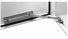
Designed for use with most standard, large mild and stainless steel enclosures to secure the door in the 90 degree open position. Door Stop Kit can be mounted at the top or bottom of the door opening after drilling two small holes in the door and enclosure. All parts are plated. Maintains UL/CSA Type 4 and Type 12 if properly installed in a Hoffman enclosure.
