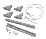
Use to mount CONCEPT<sup>TM</sup>, Networking and wall-mount enclosures to poles of various sizes and shapes. Simply attach the plated steel channel bar to the mounting holes at the back of the enclosure and wrap the stainless steel strap around the pole and through the bar. Kit includes two mounting channels, two straps suitable for 3-in. [76-mm] to 12-in. [305-mm] diameter pole and mounting hardware.
