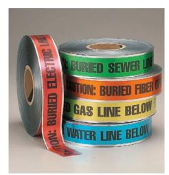
Detectable Identoline® tape minimizes time spent locating buried lines thus reducing field costs. The tape is buried 4" to 6" below the surface for maximum detectability.
