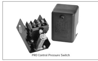
Developed and sold for use by waterwell professionals, the Furnas Brand **PRO CONTROL** pressure switch answers the professional installer's need for rugged, reliable control with no cutting corners on quality. Built for direct use on all types of pumps up to 5 Hp and for use in the control circuit of a magnetic starter (see Class 14) for larger pumps. The features of **PRO CONTROL** make it standard equipment on some of the world's finest pumps.
