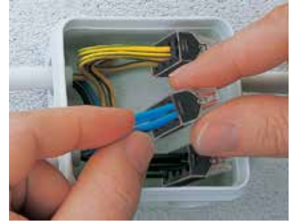
Wire Removal Solid - Pull & Twist; Remove wire Stranded - Cut Wire; Discard connector Restrip conductor and insert into new connector
