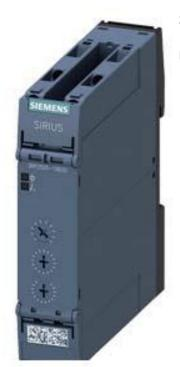
TIME RELAY, MULTI-FUNCTION, 2 CO CONTACTS, 27 FUNCTIONS, 7 TIME SET. RANGES, (1, 10, 100)s 10MIN; (1,10,100) HR 24V AC/DC AT AC 50/60HZ, LED, SCREW TERMINAL
