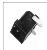
30-370-2.1 2.1 mm pin, 30-370-2.5 2.5 mm pin, PC mount coax power jack, switched circuit.
