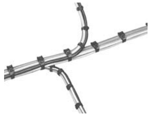
Sample cable tie installations
