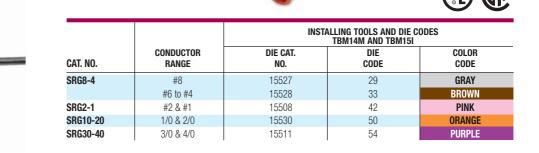
Secures signal reference grid wire to raised-floor support posts.
