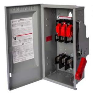
Siemens Low Voltage Circuit Protection Heavy Duty Safety Switches. Type: ENCLOSED, SAFETY SWITCH Std: CSA V. Rating: 600V A. Rating: 30 A Wattage: 3W No. Of Poles: 3P F. Rating: 60Hz Action: SINGLE THROW Material: STEEL Enclosure: TYPE 1. 2-3 point mounting holes. O. Cycles: 10000 O. Temperature: (-20F-120F) AMBIENT TEMPERATURE Environmental Conditions: INDOOR
