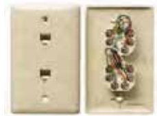
1-Gang Plate, Duplex RJ11 Jacks, 6-Position, 6-Conductor, Screw Terminations
