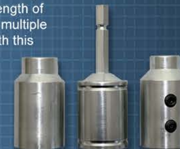
7/16" nut driver for 1/4" rod 9/16" nut driver for 3/8" rod
