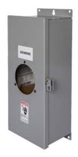
Siemens Low Voltage Molded Case Circuit Breakers Sentron Molded Case Circuit Breakers - Enclosed Circuit Breakers are Circuit Protection Molded Case Circuit Breakers. Sub Brand: SENTRON Type: MD6 Std: UL V. Rating: 600V A. Rating: 800A F. Rating: 50/60Hz Frame: MD Trip Type: THERMAL MAGNETIC Interrupt Rating: 25KA No. Of Poles: 3P Enclosure: TYPE 1S L: 64 W: 32 H: 12 Operating Temperature: (-25C -- 75C) AMBIENT TEMPERATURE
