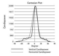
Nema type: 4H x 4V Beam spread: 57 H x 70V Beam efficiency 10%: 35.0% Beam flux 10% (lumens): 5604 Maximum candela: 23300
