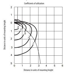
35W, low pressure sodium lamp, horizontal lamp orientation, 12' mounting height, 4,800 rated lumens.
