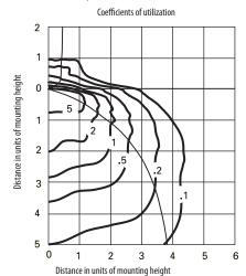
150W, high pressure sodium lamp, horizontal lamp orientation, 12' mounting height, 16,000 rated lumens.
