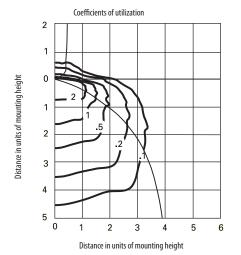
70W, high pressure sodium lamp, horizontal lamp orientation, 12' mounting height, 6,300 rated lumens.
