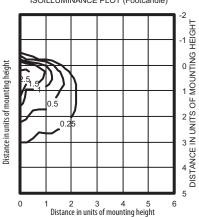
70W, metal halide lamp, horizontal lamp orientation, 10  $^{\circ}$ mounting height, 5,200 rated lumens.
