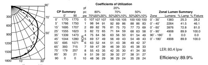
\*The LER (Luminaire Efficacy Rating) is the lumens per watt rating for this fixture. It is used to compare the energy efficiency of various products. This photometric report is based upon IES testing procedures, as stated in LM-41-1998. The reported lumen rating is based upon lamp manufacturer's published lumen output for the cold spot temperature measured during lamp calibration.
