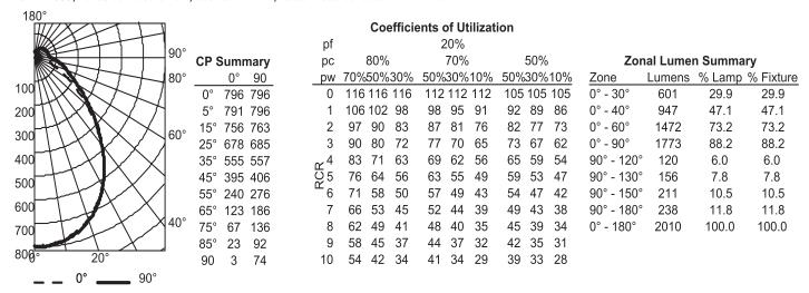
LBL4 LP835, 4050.9 delivered lumens, test no. LTL22675, tested in accordance to IESNA LM-79.
