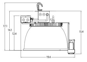
PENDANT MOUNT W/ MOTION SENSOR \*shown with optional cast hook
