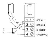
If the block is at either end of the bus, connect a terminating resistor of the appropriate type (see the System and Communications User's Manual for details) across its Serial 1 and Serial 2 terminals.
