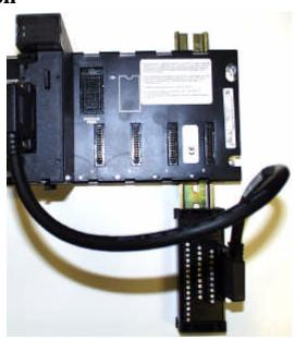
There are eight new right angle cables for the high density Series 90-30 I/O modules and Terminal Block Quick Connect. Two cables, the IC693CBL327 (**left side**) and IC693CBL328 (**right side**), have one connector on one end of the cable and finished wires on the other end. These cables are replacements for IC693CBL315 which has been obsoleted. The pin outs are the same as the old IC693CBL315.
