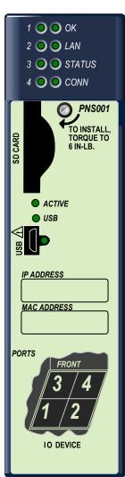
**Note:** Under certain ambient operating temperatures, the PROFINET Scanner could momentarily display the over temperature pattern during power up, while it is calibrating its thermal protection functions. This indication can be ignored. For details, see "Microprocessor Over Temperature" in the *PACSystems RX3i PROFINET Scanner Manual*, GFK-2737.
