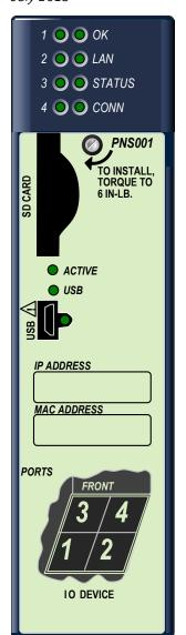
The PACSystems\* RX3i PROFINET Scanner (PNS) module, IC695PNS001, connects a remote universal RX3i I/O rack of Series 90-30 or RX3i modules to a PROFINET IO-Controller. The PROFINET Scanner scans the modules in its rack, retrieving input data and providing output data, and exchanges that data on the PROFINET IO LAN at the configured production rate.
