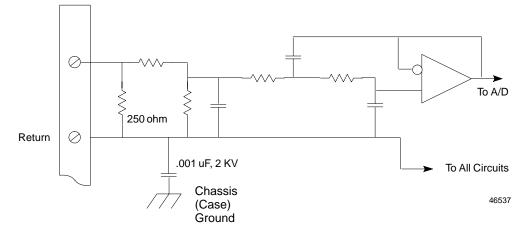
The module stores the most recent 16 samples for each channel in a buffer. The outputs of the buffer amplifiers are sequentially connected by an analog multiplexer to a 16-bit A/D converter. All channels are converted approximately once every millisecond.. The input span of the A/D is fixed, presenting binary values of 0 to 65535 for 0 to 25 milliAmps, with one LSB = 0.38 microAmps.
