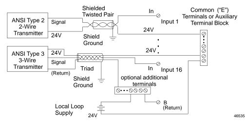
If the module is installed on an LO Terminal Block with Box Terminals or Barrier Terminals, an Auxiliary Terminal Block can be used as shown to provide the additional wiring terminals. For the LO Terminal Block with Wire to Board Connectors, external connection points are usually preferred, although an Auxiliary Terminal Block can be used. Auxiliary Terminal Blocks have all terminals connected together internally.
