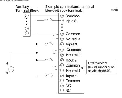
For an I/O Terminal Block with Barrier Terminals or an I/O Terminal Block with Wire to Board Connectors, an Auxiliary Terminal Block with Barrier Terminals might be connected as shown in the following example.
