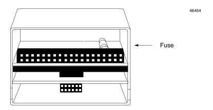
Carefully pry the fuse upward to remove it, taking care not to damage any components in the module. Place the new fuse in position and press it into the holder.
