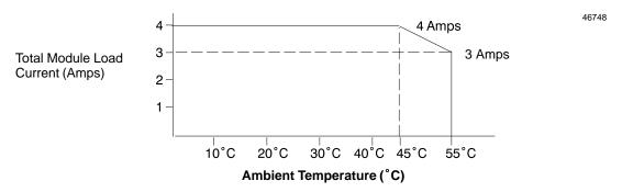
Each output on this module is capable of transiently conducting a surge current that is much greater than its long-term current rating.
