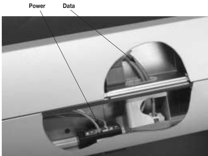
Sectioned view illustrating internal crossover capability, allowing adjacent downward facing power and data activations. Raceway profile meets or exceeds EIA/TIA bend radius requirements.
