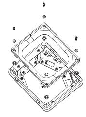
11. (S39 Series – Flush Installation) Confirm top edge of Flange is level with Floor Covering with Level or Straight Edge.
