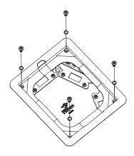
**10. (S39 Series – Flush Installation)** Top of Flange adjusted flush with Floor Covering.
