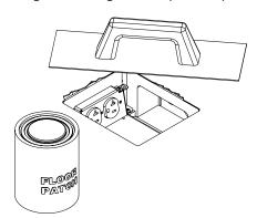
2. Install standoffs, adjusting screws, and link straps as shown.
