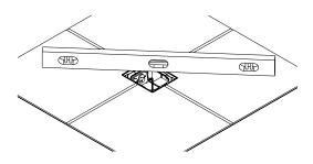
**12. (S39 Series – Flush Installation)** Seal edge of Flange with Grout or Silicone.
