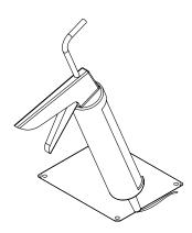
2. Place 1/8" [3.2mm] aluminum Top Plate over the Bottom Plate. Install the four Screws provided to secure the two Plates.
