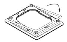
**6. (S38 Series – Flush Tile Installation)** Place flat Gasket under Trim Ring prior to positioning on concrete.
