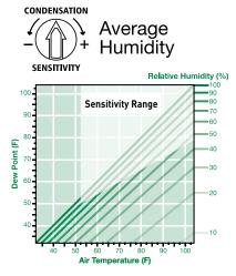
HSW is set at the factory to the most common setting. The sensitivity range on the chart shows at which point HSW will turn ON the fan or ventilation system.
