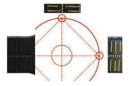
Select a hole saw that measures about 1/8" larger than the bolt to be used and drill the template at the selected easy centering divot mark.
