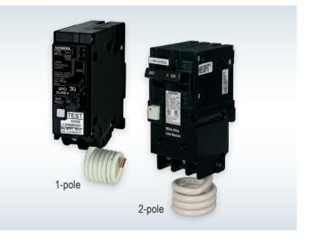
Siemens GFCI circuit breakers are UL Listed and CSA Certified as Class A devices. Current imbalances of 4-6 milliamps or more between load conductors will cause the ground fault sensor to trip the circuit breaker.
