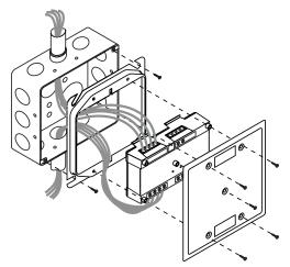
**SIGA-MCC1 and SIGA-MCC2:** mount the UIO motherboard inside a suitable GE Security enclosure with screws and washers provided. Plug the SIGA-MCC1 or SIGA-MCC2 into any available position on the motherboard and secure the module to the motherboard with the captive screws. Wiring connections are made to the terminals on the motherboard (see wiring diagram). UIO motherboard terminals are suited for #12 to #18 AWG (2.5 mm<sup>2</sup> to 0.75 mm<sup>2</sup>) wire size.
