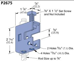
Clamp Materials: .105" (2.7) thick steel. Clamp P2675 is designed for light duty rod suspension. It also may be used with P3016-1024 or P3016-1420 nut as illustrated above for mounting insulators, etc.
