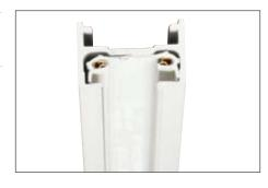
Fast Track single-circuit track enables all the Lytespots to work in tandem. It can be surface or stem mounted on ceilings, and mounted vertically or horizontally on walls, in straight runs or patterns. It can be field cut to the desired length. Capacity is 20 amps at 120V per branch circuit.
