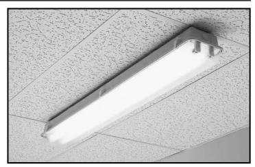
Rapid start units with cold weather ballast are for maximum 10°C ambient. Do not flush mount HO units. Should be suspended minimum 1-1/2" from surface. 248H and 296H units are for maximum 15°C ambient.
