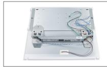
Step 1: EvokitSR is shipped with a plate covering the sensor hole. There are two wires secured to the back of the plate.
