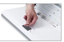
Step 3. Remove the two wires that were secured to the back of the plate.
