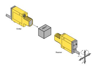
"Flooding" occurs when a portion of the sensing beam passes around the object to be sensed. "Burn-through" occurs when a portion of the emitter's light energy passes through a thin or translucent object, and is sensed by the receiver.
