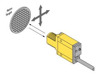
A highly reflective object may reflect enough light back to a retroreflective sensor to allow that object to slip through the beam, without being detected. This problem is called "proxing," and the following methods may be used to correct it:
