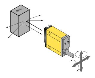
If the Alignment LED does not go OFF when the object is removed from the beam, the sensor is probably detecting light reflected from some background object. To remedy this problem:
