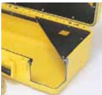
Panel mounting rings are available for Dry Boxes and Dry Cases. The ring is solvent welded in place 0.5 inch below the rim of the case. Brass threaded inserts (8-32) are embedded in the ring for rigid attachment of an instrument panel. A foamed neoprene O-ring seals the panel to the ring.
