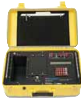
Panel mounting rings are available for Dry Boxes and Dry Cases. The ring is solvent welded in place 0.5 inch below the rim of the case. Brass threaded inserts (8-32) are embedded in the ring for rigid attachment of an instrument panel. A foamed neoprene O-ring seals the panel to the ring.
