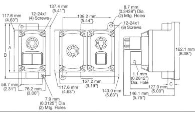
EFD/EFDB — 1-Gang Dust Cap Push Button and 1-Gang Maintained Contact Push Button
