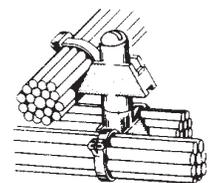
Mounting blocks permit vertical stacking and can be used in any direction. Natural nylon colour. For use in temperatures ranging from -40°C to 85°C (-40°F to 185°F).
